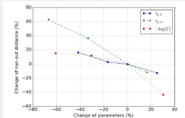
**Figure 13.** Parameter sensitivity tests for runout distance. Change of runout distance is shown with respect to the change of parameters. Parameter changes are relative to  $\tau_{y,0} = 12$  kPa,  $\tau_{y,\infty} = 3$  kPa, and  $\Gamma = 5 \times 10^{-4}$ . The runout distance is most sensitive to changes in  $\tau_{y,\infty}$ .
