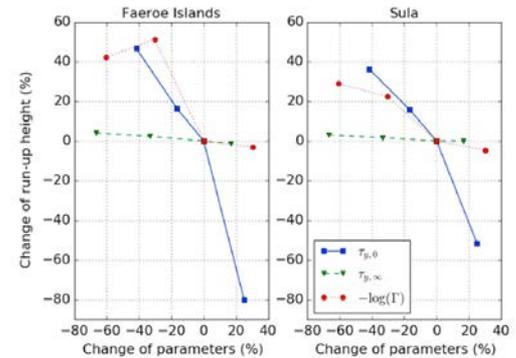
**Figure 14.** Parameter sensitivity tests for the maximum tsunami heights at two locations. The changes of the maximum tsunami height at the Faeroe Islands and Sula are shown with respect to the change of parameters. The maximum tsunami heights in both locations are rather sensitive to the choice of  $\tau_{y,0}$  and  $\Gamma$ .
