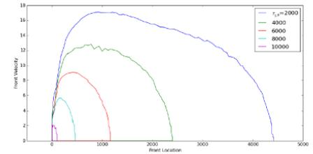
Figure 4.35: Maximum landslide plug velocities for  $f=5 \cdot 10^{-4}$ , with  $\tau_{y,0} = 2 \text{ kPa}$  and variable  $\tau_{y,0}$ .
