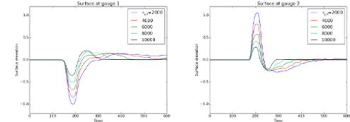
Figure 4.36: Time series of the induced tsunamis due to a Bingham fluid with different initial yield strengths  $\tau_{y,0}$ . Gauge 1 and 2 are located at  $x = -5000$  (behind the landslide) and  $x = 15000$  (in front of the landslide), respectively.
